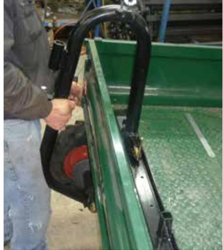
3. When the frame is in place mark the position of the mounting frame holes in the bed. Check underneath for wires, pipes and clearance. You can now drill and bolt through the bed and secure the mounting frame using the plates provided.
