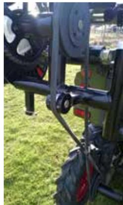
3. Tension the belt by attaching the stay bar from the wheel arm to the winder and securing with a wing nut screw.
