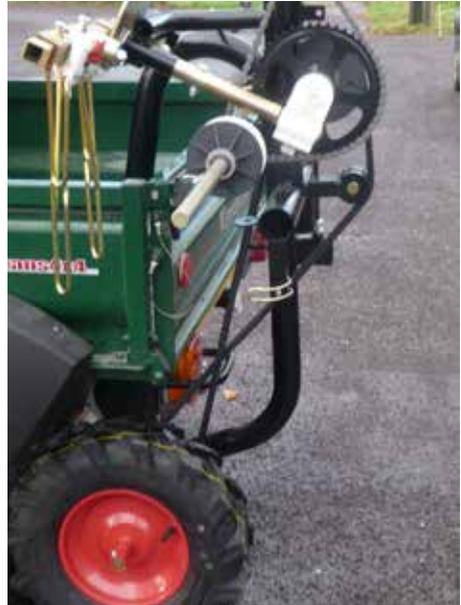
6. The belt position is crossed in a figure of eight between the Top Pulley and Wheel Arm Pulley.
