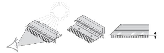
The best hollow-grind: For cattle and horse blades between this:  $5-15\mu m$  For PET blades between this:  $0-5\mu m$
