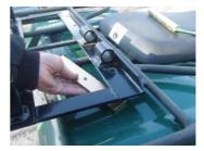
Attach the yellow winder to the wheel arm and swing into working position. Rotate the mechanism fully to check that there is clearance on all moving parts between the winder and ATV.
