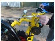
All adjustments are preset before delivery however after some use it may be necessary to adjust the belt tension. To do this move the 17mm bolt on the wheel arm up to tighten or down to slacken.
