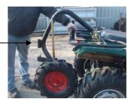
Once the required position is reached, secure the frame with the clamping plates and lightly tighten. Try to clamp the frame onto the strongest parts of the ATV pannier.
